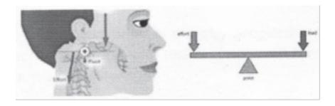
Following is the example of class II lever which is used by our body.
